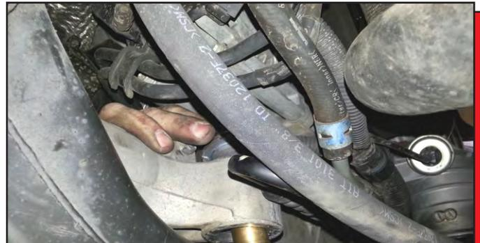
**Driver side:** The rack will move toward the passenger side and forward just enough to remove the bushing.
