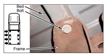
Remove four bed bolts from frame passenger side.
