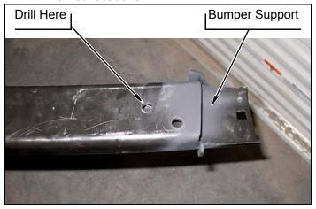
**m.** Install bumper support onto two *kit* **brackets** (bumper, rear) with four *kit* **bolts** (1/2"-13 x 3"), eight *kit* **washers** (1/2" SAE) and four *kit* **nuts** (1/2"-13 Stover). DO NOT TIGHTEN.
