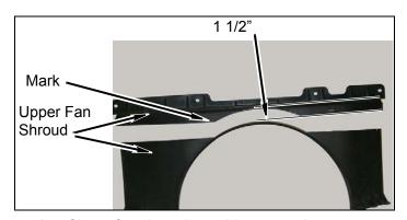
b. Clamp fan shroud on table top as shown.
