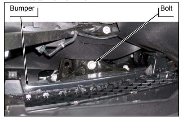
g. Install two kit brackets (bumper, front, support) onto two cab mounts with four kit bolts (7/16"-14 x 1-1/2"), eight kit washers (7/16" SAE) and four kit nuts (7/16"-14 Stover). DO NOT TIGHTEN.
