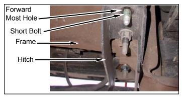
u. Install kit brackets (rear bumper) and hitch on frame with two long bolts, two kit washers (1-1/2 x 2-1/2 rectangular), two kit washers (14mm), into two kit nuts (14mm nylock).
