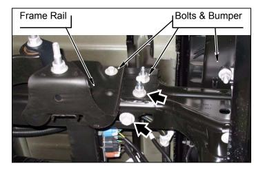
c. If equipped with a trailer hitch, remove two short and two long bolts from hitch and frame.
