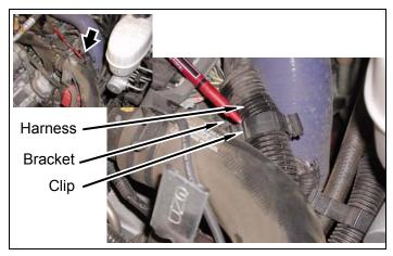
Remove two clips and harness from cover and inner fender.
