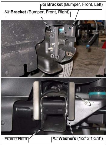
c. Install frame bracket onto kit brackets (bumper, front) with two kit sleeves (.75" OD x .532" ID x 3.35" L), four kit bolts (1/2"-13 x 5-1/2"), eight kit washers (1/2" SAE) and four kit nuts (1/2"-13 Stover). DO NOT TIGHTEN.
