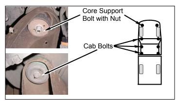
b. Remove core support bolt, nut, and three cab bolts from passenger side cab.
