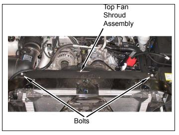
e. Install top fan shroud on bottom fan shroud with four pop-ups. Check fan to shroud clearance. Ensure gap is the same all around shroud.
