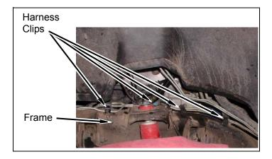
d. If possible, install two brake lines in two sets of clips. If brake lines will not fit back into position, wrap lines with two kit **zip ties** individually, and then secure the lines together with one kit **zip tie** as a bundle.
