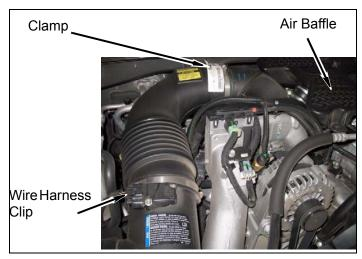
b. Rotate air intake assembly away from engine and towards fender while pulling the air box up and out of rubber grommets on fender.
