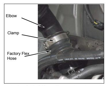
b. Install *kit* **3" Hump Hose** on lower intercooler pipe using factory clamp.
