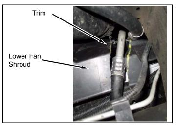
b. Remove bottom lip from lower fan shroud in five places as shown.
