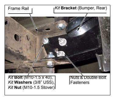
s. Install kit **bracket**, hitch spacer and two kit **blocks**, lift (3" x 2" large hole) as shown, on rear bumper and hitch with two kit **bolts** (14mm x 110mm) and two kit **washers** (14mm). Do not tighten.
