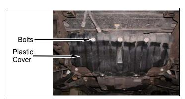
b. Remove plastic cover from push clip, lower radiator hose and vehicle.
