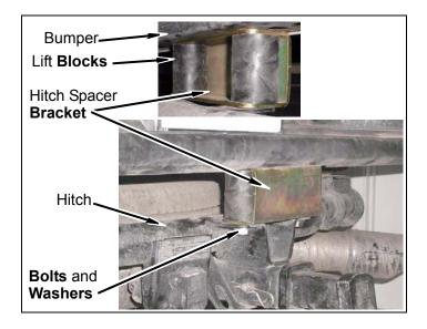
t. Install hitch on frame with two short bolts and nuts. Use forward most hole in hitch.
