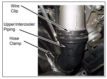
b. Remove intercooler pipe and hose from vehicle
