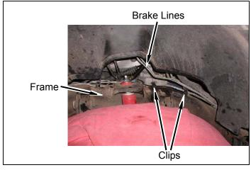
e. If possible, install harness in clip on frame driver side.
