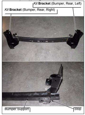
**f.** Mark and cut left and right of bumper as shown.
