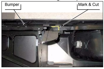
g. Install bumper support and two kit brackets (bumper, rear) onto bumper with two O.E. carriage bolts and six nuts. Snug, but DO NOT TIGHTEN.
