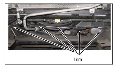
c. Position bottom fan shroud in vehicle and rest below lower core support.
