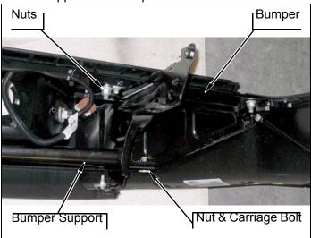
**d.** Cut two brackets and remove from bumper support as shown.
