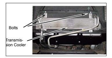
c. If necessary, carefully bend hard line and secure with kit **zip tie**.
