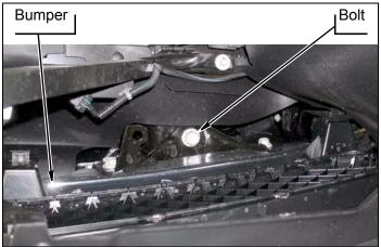
**d.** Remove four nuts, two double-bolt fasteners and two frame brackets from two frame horns.
