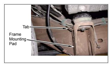
c. Install the front parking brake cable housing as shown.
