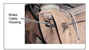
Install two ground wires on frame mounting pad with bolt. Connect front and rear brake cables. Remove clamps from rear cable.
