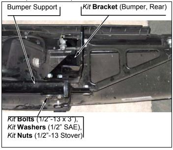
**n.** Install bumper support and two *kit* **brackets** (bumper, rear) onto bumper with two O.E. carriage bolts and six nuts. DO NOT TIGHTEN.
