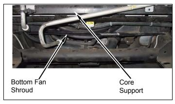
d. Install upper fan shroud assembly on core support with two bolts. Do not tighten.
