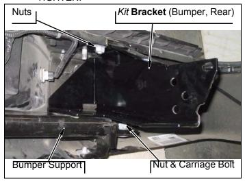
h. Install bumper onto frame rails with two O.E. double-bolt fasteners, two nuts, two kit bolts (M10-1.5 x 40), four kit washers (3/8" USS) and two kit nuts (M10-1.5 Stover). Snug, but DO NOT TIGHTEN.
