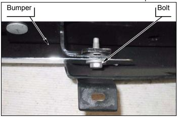
**c.** Remove six nuts, two carriage bolts and bumper support from bumper.
