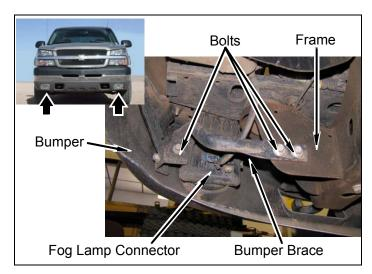
**c.** Remove two bolts and bumper from frame horns.
