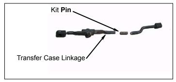
d. Install transfer case linkage on transfer case shift arm and shift lever with two clips.
