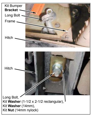
v. Adjust bumper to bed clearance using measurements taken earlier and tighten hitch bolts first then remaining bolts and nuts to 55 lb-ft.
