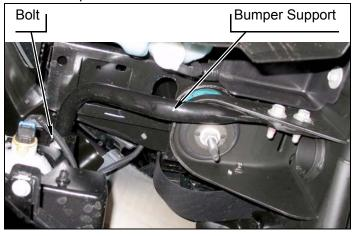
**f.** Install bumper onto frame brackets with two O.E. bolts. DO NOT TIGHTEN.
