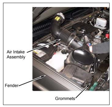
b. Tighten clamp on air intake assembly. Install wire harness clip on sensor.
