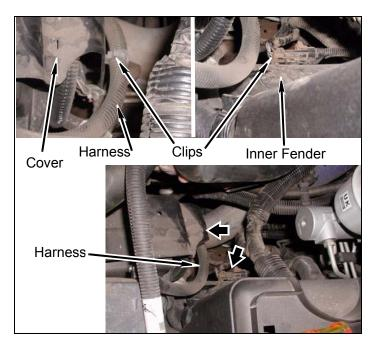
7. Wiring harnesses and power steering drivers side
