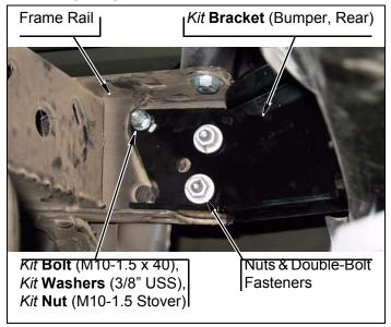
i. Mark eight holes through two *kit* **brackets** (bumper, rear) onto bumper support.
