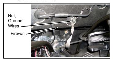
**b.** Remove clip and wiring harness from fire wall.
