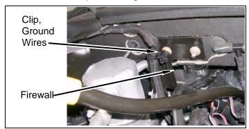
**c. Driver Side**: Remove two nuts and vacuum control module from fire wall.
