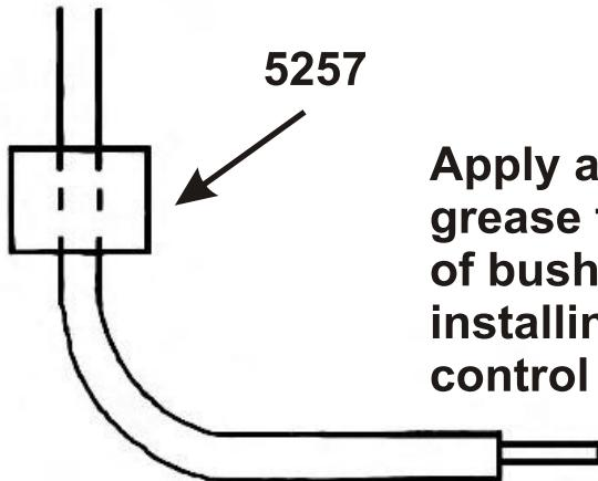
**Apply a light coat of grease on the sway bar bushing I.D. & sway bar at bushing contact area.**
