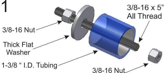
Parts needed to make a simple puller to remove old rubber bushings from rack & pinion can found at local hardware store, around the house, grandpa's old toolbox or a friend or neighbor.
