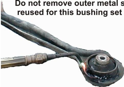
Apply light heat evenly around the outside of the outer metal shell, just enough to break the bond with the rubber. When you see light smoke coming from the sides of the bushing the bond should be broken. At no time should there be any flames coming from the rubber, if there are any flames, you need to back off with the heat. Just push the old rubber and inner metal sleeve out. Let the outer metal shell cool before cleaning the inside.
