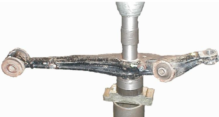
A hydraulic press was used to remove the original bushing, including the outer metal casing the rubber is bonded to. The inside diameter of the control arm is  $\text{Ø } 36\text{mm}$  (1.417"). Go about .050" smaller when pressing out the bushing.
