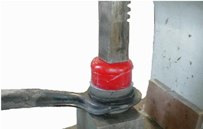
Let metal shell cool before cleaning inside. Remove any burrs and sharp edges before applying grease. Clean the hole/barrel in the control arm that you just removed the bushing from. Lubricate the inside of the hole/barrel. Grease all sides of the bushing that contact metal. Press in the Energy Suspension bushing. Grease the sleeve and press into the bushing.
