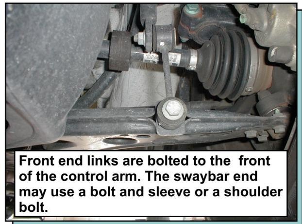
Front end links are bolted to the front of the control arm. The swaybar end may use a bolt and sleeve or a shoulder bolt.
