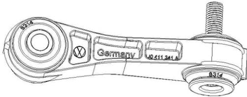
This link uses P/N 8314 and sleeve # 15.10.442.39. Must reuse O.E. shoulder bolt at bar end.
