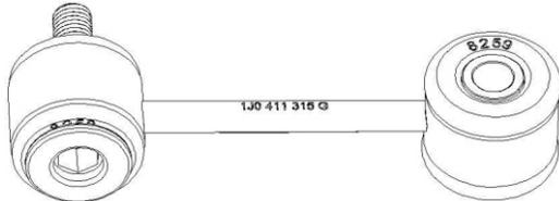
This link uses P/N 8258, 8259 and sleeve # 15.10.442.39. Must reuse O.E. shoulder bolt at bar end.
