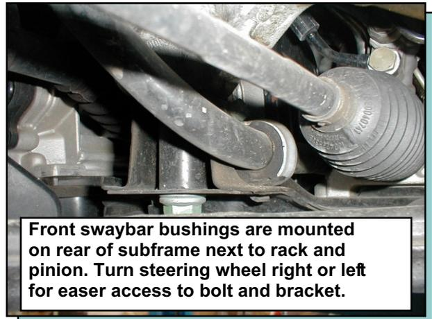
Front swaybar bushings are mounted on rear of subframe next to rack and pinion. Turn steering wheel right or left for easier access to bolt and bracket.
