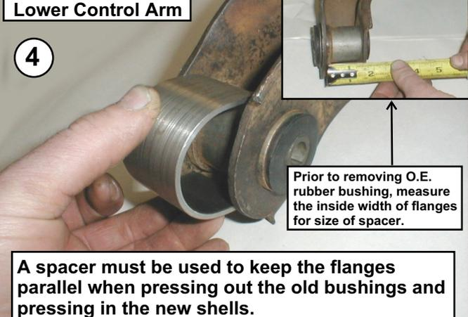
Prior to removing O.E. rubber bushing, measure the inside width of flanges for size of spacer.
