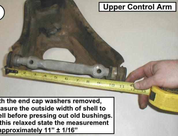
With the end cap washers removed, measure the outside width of shell to shell before pressing out old bushings. At this relaxed state the measurement is approximately 11" ± 1/16"
