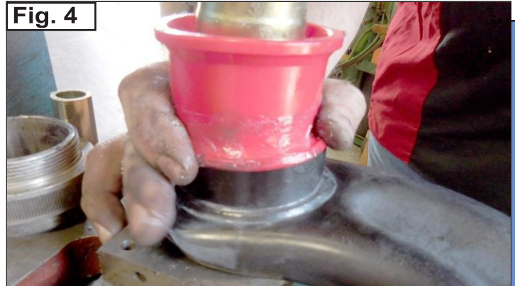
Squeeze the leading edge of bushing 03P03585 to help get it started into the eye. Then press in the inner metal sleeve 15.10.568.39.
