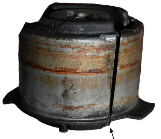
Outer metal shell cut lengthwise with a metal blade
