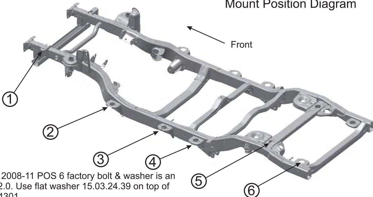
**NOTE:** 2008-11 POS 6 factory bolt & washer is an M14 x 2.0. Use flat washer 15.03.24.39 on top of mount 4301.
