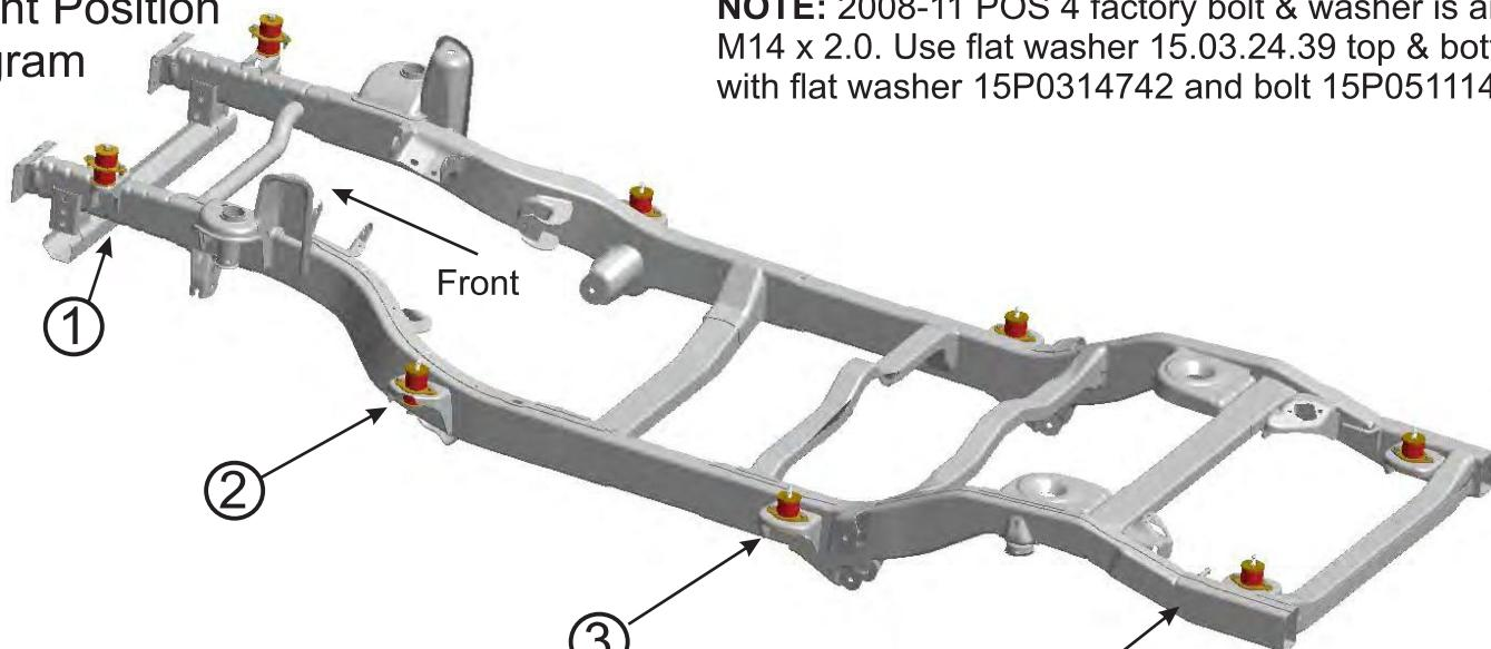
**NOTE:** 2008-11 POS 4 factory bolt & washer is an M14 x 2.0. Use flat washer 15.03.24.39 top & bottom with flat washer 15P0314742 and bolt 15P0511140.
