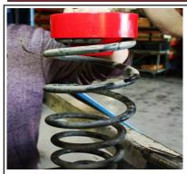
Install your new polyurethane coil isolator in place of the stock rubber isolator and ensure that it is properly seated.
