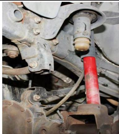
Install your new polyurethane coil isolator in place of the stock rubber isolator and ensure that it is properly seated.
