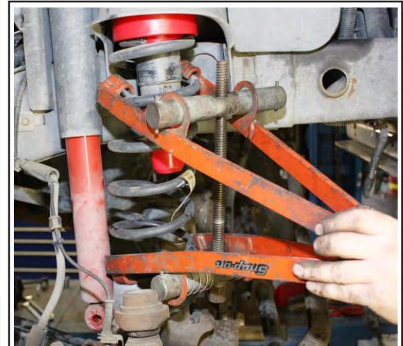
Install the coil springs on their designated sides of the vehicle. A spring compressor may be needed to ease the installation of the spring. Lower the vehicle to ride height. Reconnect the endlinks, lower shock mount, and ABS wires and torque bolts to factory specs. It is recommended to have your vehicle aligned after the installation of these parts.
