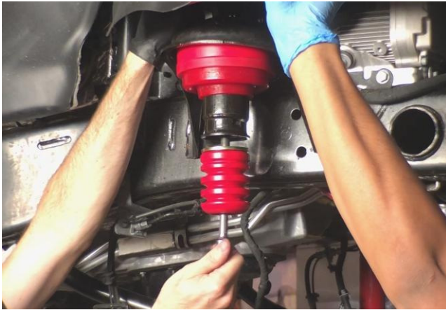
Image 5. Front Jounce Bumper Installation
