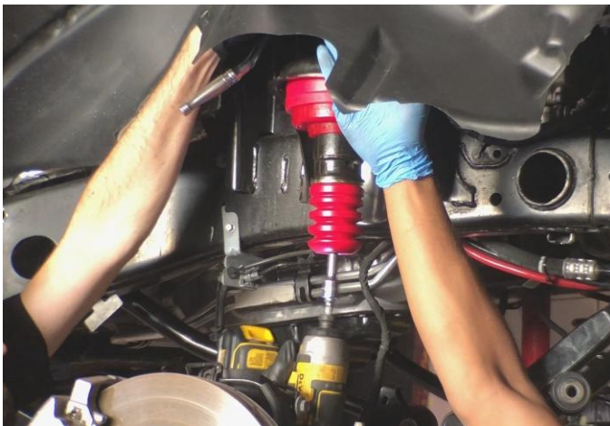
Image 6. Front Jounce Bumper Bolt Tightening
