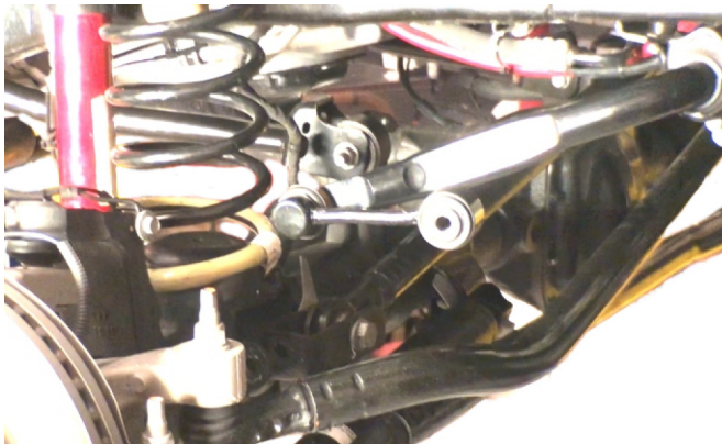
Image 2. Swaybar Link Detached
