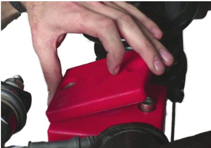
Image 9. Jounce Bumper Spacer Installation
