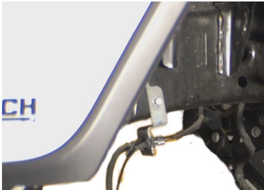
Image 1. ABS wire at frame
