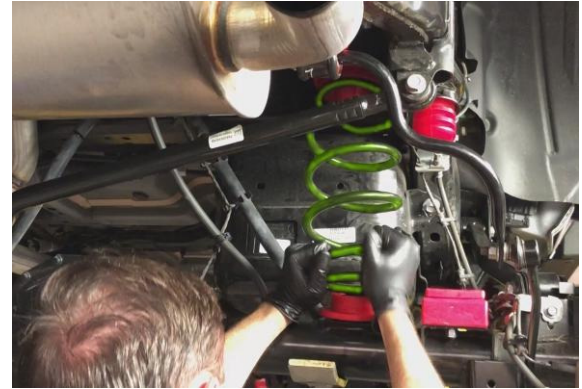
Image 9. Rear Spring Installation
