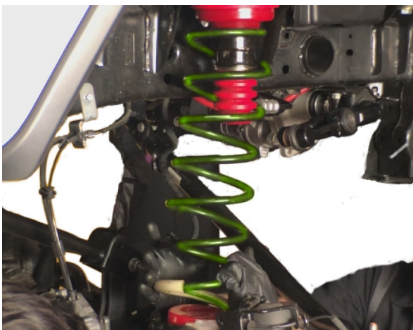
Image 6. Coil Spring Installation
