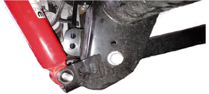
Image 3. New and Existing Hole in Sway Bar Mounting Tab
