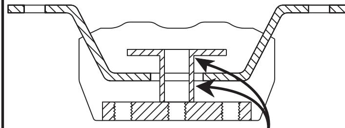
Side view (cutaway) showing safety interlock
