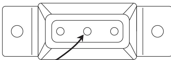
This hole is not used. (Center hole is for manufacturing purposes.)
