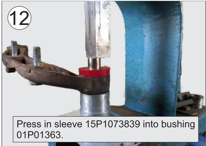
Press in sleeve 15P1073839 into bushing 01P01363.
