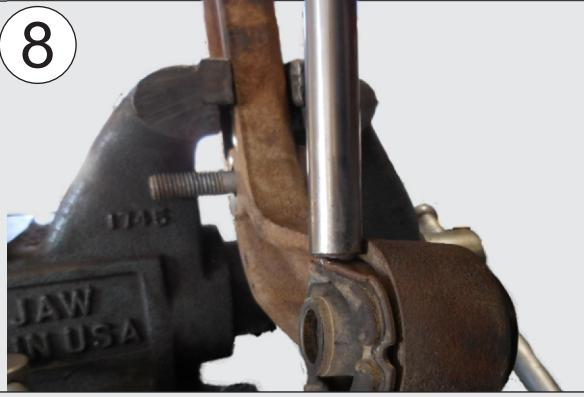
Flip the differential carrier bracket over and fold over the flange 180° from the other side.
