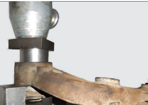
Support the differential carrier bracket next to folded flanges and press out metal shell. Differential carrier bracket I.D. Is Ø1.835
