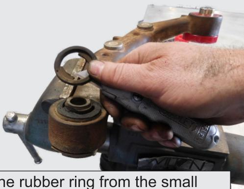
Cut the rubber ring from the small side of the factory bushing.
