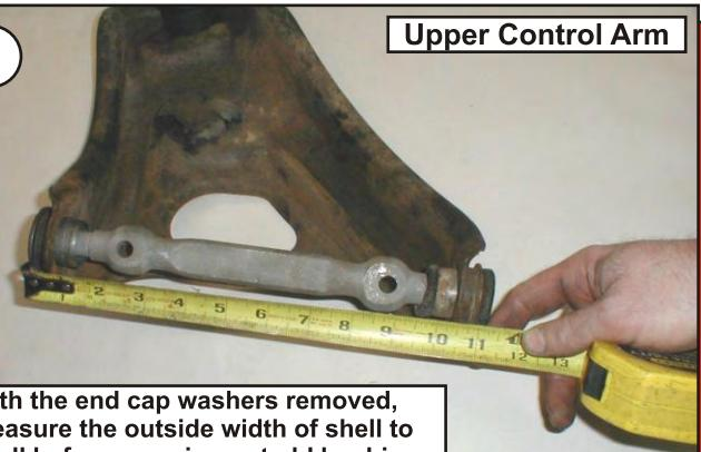
With the end cap washers removed, measure the outside width of shell to shell before pressing out old bushings. At this relaxed state the measurement is approximately  $11" \pm 1/16"$
