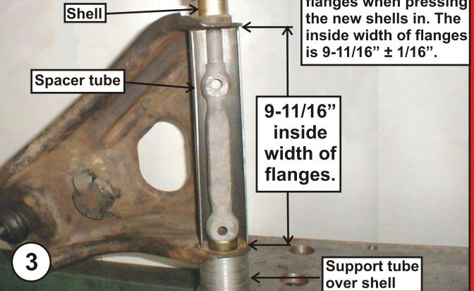
The upper arm needs support between the flanges when pressing the new shells in. The inside width of flanges is  $9-11/16" \pm 1/16"$ .
