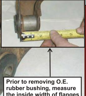
Prior to removing O.E. rubber bushing, measure the inside width of flanges for size of spacer.
