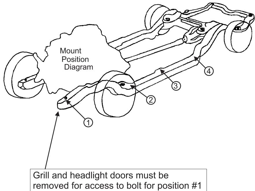
Install mounts one side at a time with bolts on other side loosened only.
