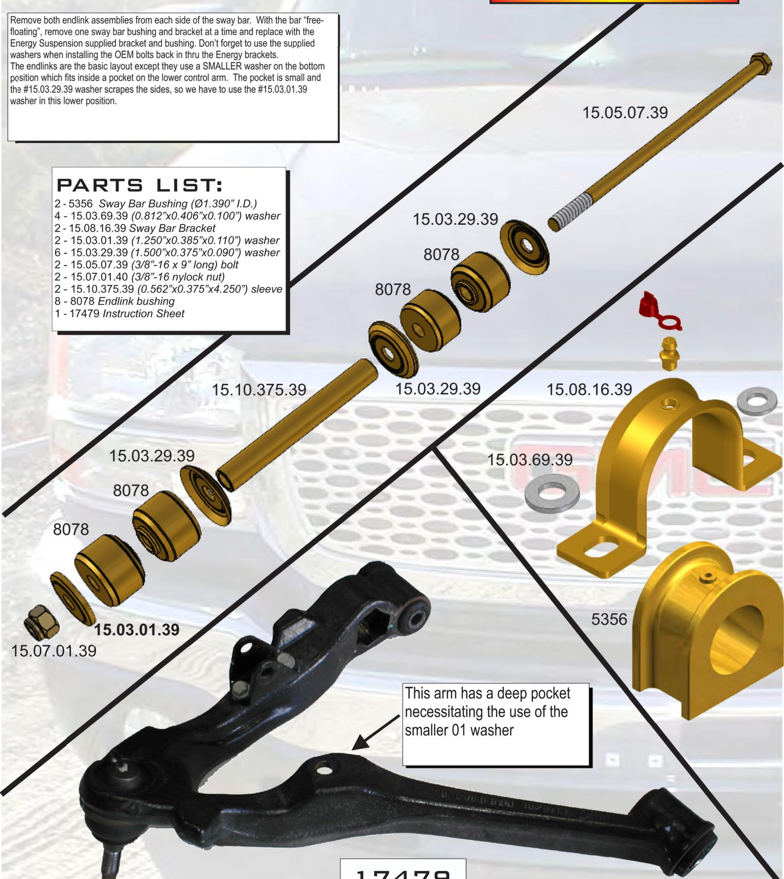
This arm has a deep pocket necessitating the use of the smaller 01 washer
