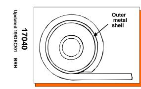
**Note:** When a sleeve is not used, apply a light coat of grease to the original shoulder bolt. **Remember:** Most spring eyes have an outer metal shell. Some shackles are this way as well. The outer shell must be removed.
