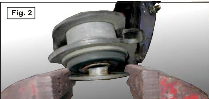
Cam Bolt style Bushing's use a special washer on each end of the sleeve. To remove cap washers on upper or lower control arms, clamp cap washer in vice and wiggle arm back and forth. When new washers are not supplied in kit, originals must be reused.
