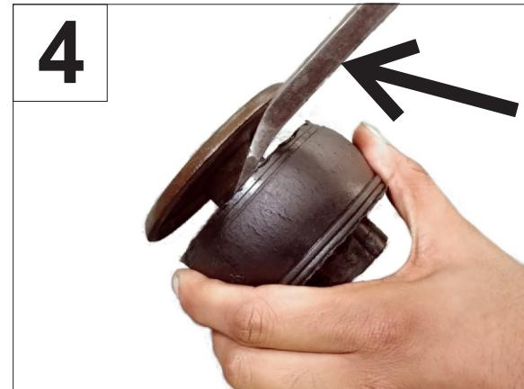
Use spray lube and pry-bar to remove old rubber body mount from O.E. metal.
