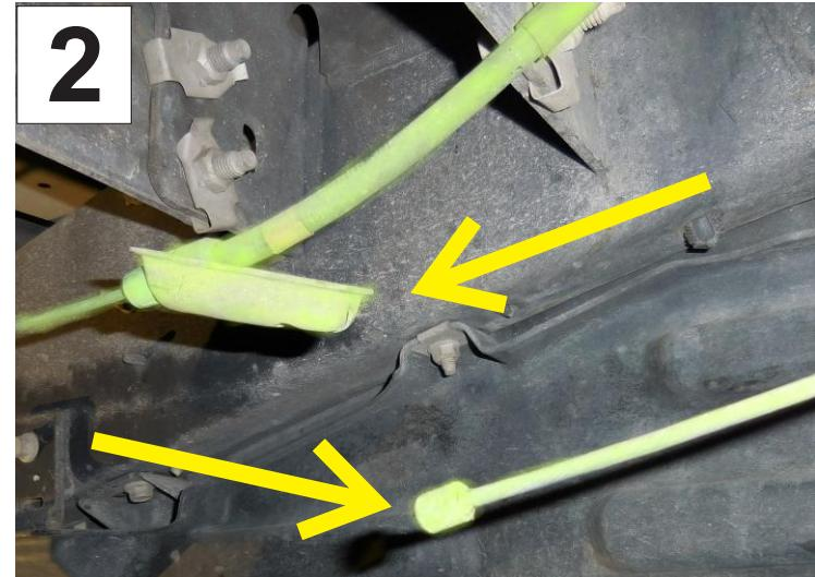
Unhook park brake cable located near rear main spring eye on driver's side.
