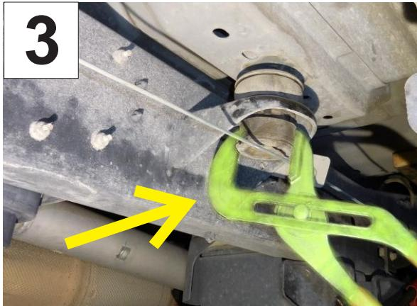
Use large tongue and groove pliers to separate bottom half of body mount.
