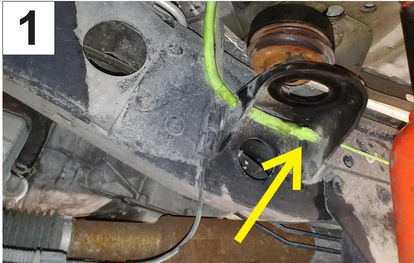
Release park brake cable clip from position 2 frame perch on driver's side before lifting body.
